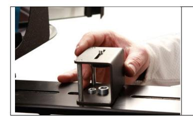
The base plate has slots that assist front to back adjustments.
