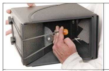
For shipping and storage, place the removable mirror against the beam splitter to protect both.
